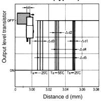
$\begin{array}{l} \mathsf{V}_{cc} = 12 \; \mathsf{V} \\ \mathsf{No.} \; of \; repetitions: 20 \\ \Delta d1 = 0.002 \; mm \\ \Delta d2 = 0.004 \; mm \\ \Delta d3 = 0.005 \; mm \\ \Delta d4 = 0.02 \; mm \\ \Delta d5 = 0.04 \; mm \end{array}$
