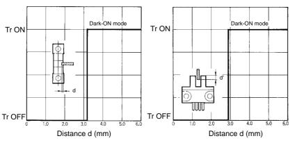
Repeated Sensing Position Characteristics (Typical)
